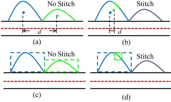
Fig. 6. Illustration of our two high-level geometric features/metrics. The blue and green curves represent two connecting patches. The red dash line represents the backbone.
