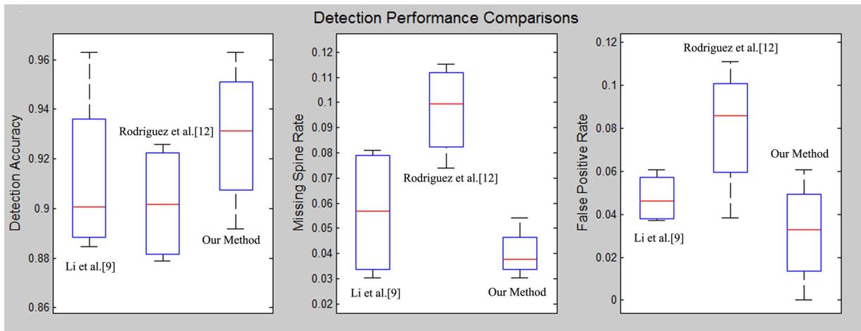
Fig. 8. Detection performance comparisons between our approach and the two chosen spine detection algorithms [13], [16]. The Y axis of the three panels (from left to right) is “detection accuracy”, “missing spine rate”, and “false positive rate”, respectively.
