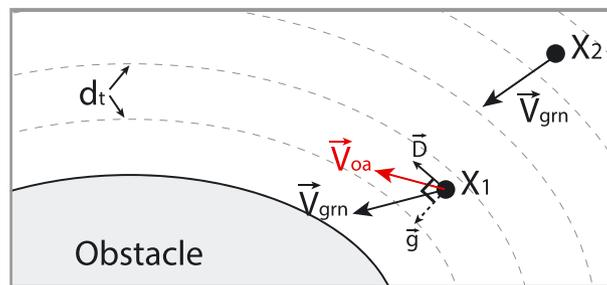
Figure 5. An illustration of computing the obstacle-avoidance velocity.
