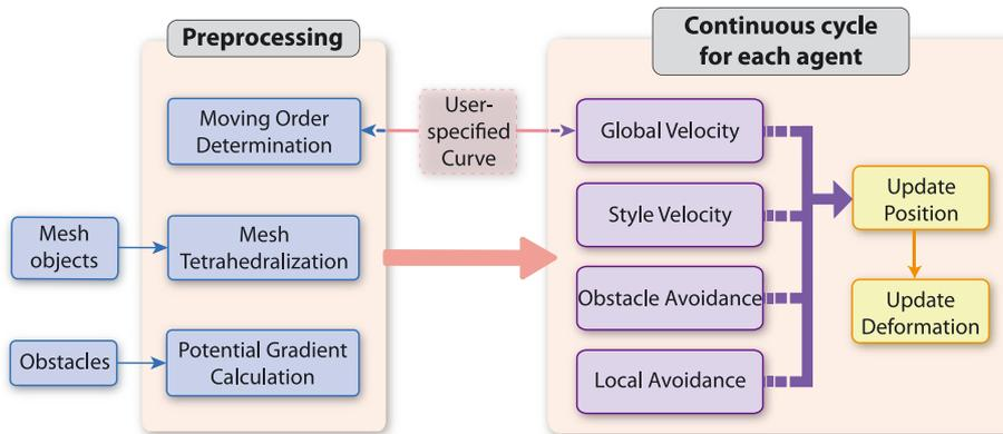
**Figure 2.** The pipeline of the proposed approach.
