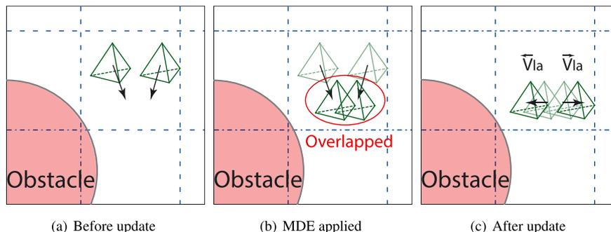
Figure 6. An illustrative example of the minimum distance enforcement rule.
