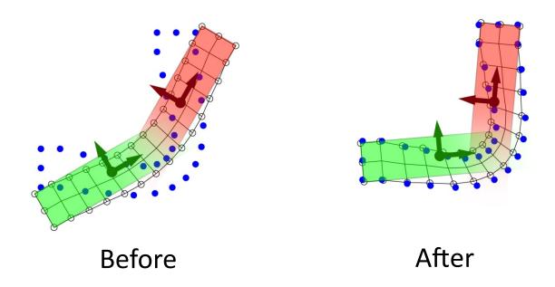
• The residual for bone  $\hat{j}$   $E^t = \left\| v_i^t - \sum_{j=1}^{|B|} w_{ij} (R_j^t p_i + T_j^t) \right\|^2$
