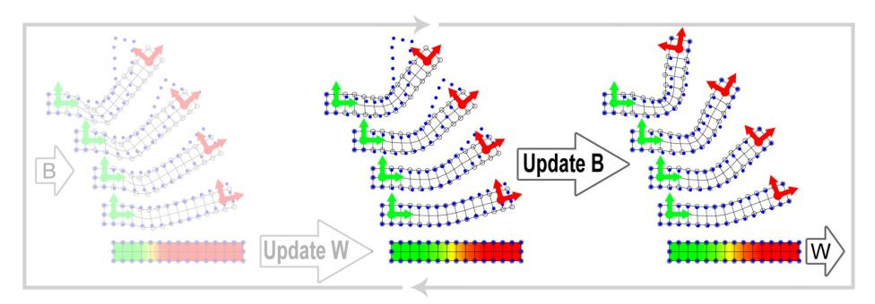
No blending (rigid binding): each vertex is driven by exactly one bone
