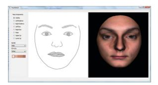
Figure 2: A snapshot of our running system that consists of three main panels. Left: parameter setting for a user to select face component and texture information. Middle: a sketching interface for a user to draw a free-form face. Right: the resulting photorealistic 3D face.
