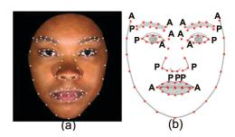
Figure 3: (a): 83 feature point locations. (b): the Anchor points (A) and the Pivot points (P) on the rendered portrait.
