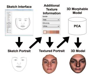
Figure 1: The schematic view of our system. It consists of three main components: a face sketching interface, automated facial texture generation, and 3D face construction.
