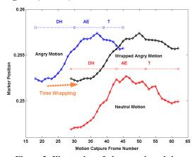
Figure 3: Illustration of phoneme-based timewarping for the Y position of a particular marker. Although the phoneme timings are different, the warped motion (black) is strictly frame aligned with neutral data (red).
