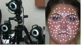
Figure 2: Illustration of motion data acquisition. The left shows the cameras of the motion capture system. The right shows the markers used in the data acquisition stage.
