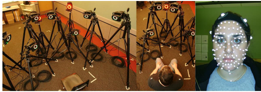
Figure 1: Snapshots of the used motion capture system. The left two panels show the system, and the right panel shows the used facial marker configuration.
