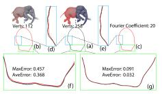
Figure 16. The high-resolution curve (a) in polygon mesh reduced to (b) with large accuracy lose in (d), (f). But Fourier series representation (c) keep high realism with sharply decreasing data-size.
