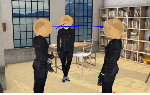
Figure 3: Visualization of the GTV computation process. The resulting Direction-of-Focus (DFoc) is depicted as a blue line.
