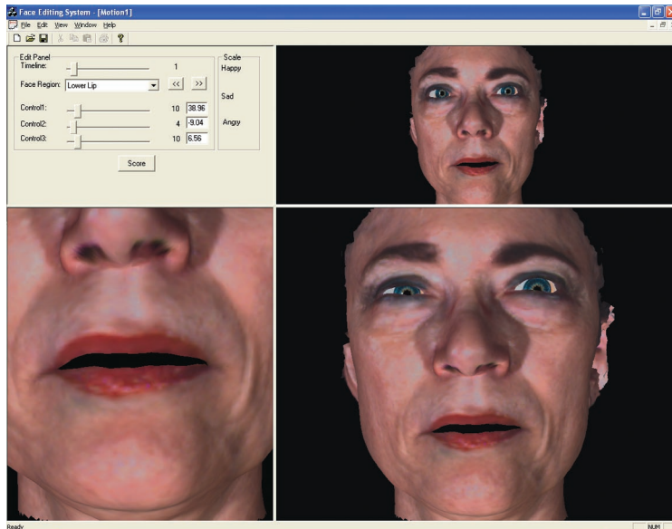
Figure 10. Our system in action. The top-left panel is a blendshape control window in which users can select a facial region and move its weight sliders, the bottom-left panel displays the edited results without weight propagation, the top-right panel displays the original facial motion capture sequence, and the bottom-right panel displays the edited facial-motion sequence (the final output) after constrained weight propagation is applied.
