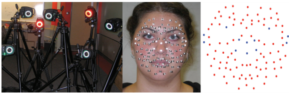
Figure 2: The left shows a facial motion capture system, the middle is a snapshot of the captured actress. In the right panel, blue and red points represent the 102 captured markers, where the red points are the 90 markers used for this work.
