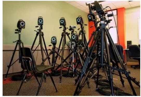
Fig. 2. Vicon motion capture system used in the study to capture the trajectories of the markers depicted in Fig. 1.
