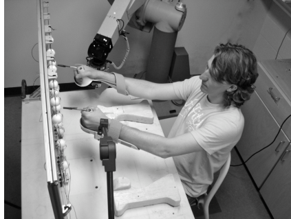
Figure 1. A picture of the experiment set up. Right-handed participants were seated in front of a target array and placed their arms in forearm splints. The right splint was attached to the Puma-560 robot (Stäubli Unimation, Inc.). Optical encoders in each of the robot's six joints allowed monitoring of the position and orientation of the splint, while a six-axis force-torque sensor (resolution 0.25N) on the end of the robot measured any forces and torques applied. The left splint was attached to the position digitizer (MicroScribe-3DLX, Immersion Corp.), which could measure arbitrary trajectories for the left forearm while applying minimal resistance to movement.
