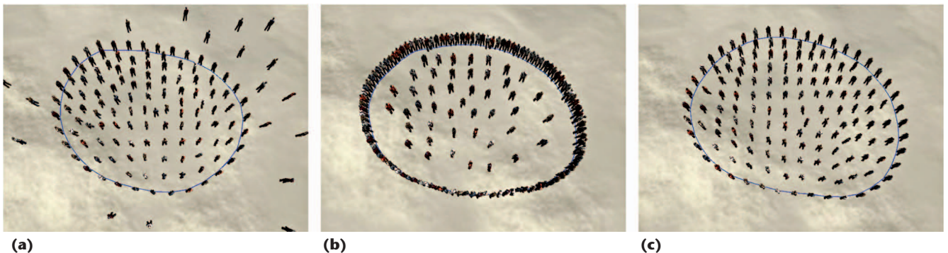
Figure 5. Sampling-unit optimization. (a) An overly large sampling unit gives the template fewer points than agents. (b) An overly small sampling unit clusters too many agents on the boundaries. (c) Our adaptive sampling algorithm evaluates the unit for an optimal configuration.
