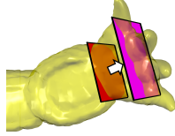
Figure 9: The cage is refined by pushing its vertices outward to bound the input model at a distance of \Delta , while keeping a minimal change on the normals of all the cage triangles.
