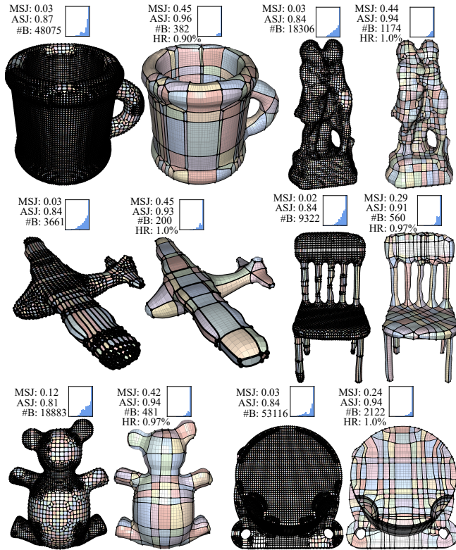
Fig. 9. Simplified results (right) on meshes (left) generated with the octree-based method [MeshGems 2015].
