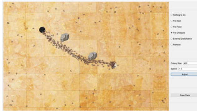
FIGURE 15 An interactive simulator built upon our motion controller. The ant colony is controlled in real time by changing the motion scenario or modifying parameters of the ant colony
