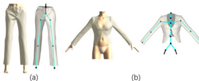
FIGURE 2 The cyan bones are taken into account in the subsequent fitting process, and these bones lie approximately at the center of the corresponding garment parts
