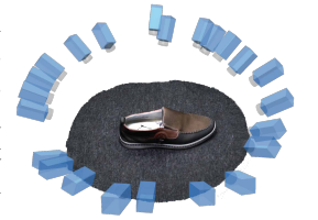
Figure 7: The camera's trajectory for the upper half of the shoe.
