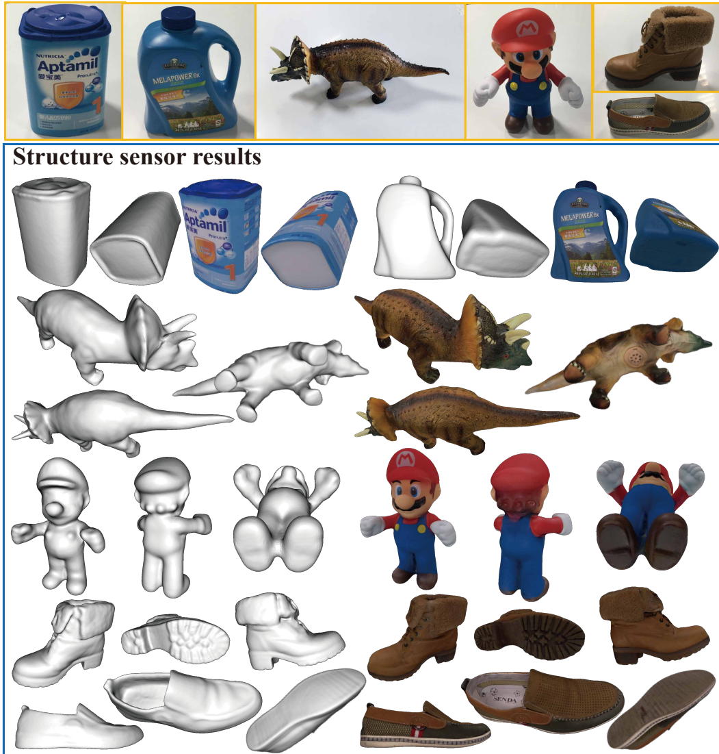
Figure 16: Our system can produce high-quality 3D reconstruction for various objects using Occipital structure sensor. It is robust for geometric-complex items like the toy dinosaur and various shoes. The photometric metric further improves the texture quality. Even the ingredient information on the formula canister is legible.
