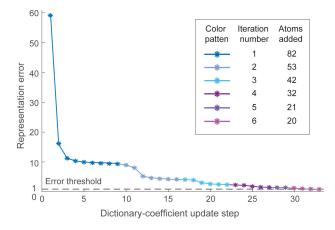
Fig. 7. The convergence of our adaptive dictionary learning algorithm. The curve segment in one color represents one iteration (i.e., one joint dictionary-coefficients optimization process after adaptively adding atoms to the dictionary). One point means the representation error after one dictionary-coefficient update step.
