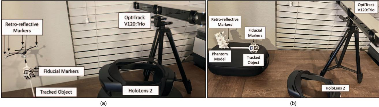
Figure 2. Experimental setup to evaluate the accuracy of the proposed surgical navigation system during (a) tracking and (b) alignment.
