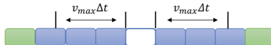
FIGURE 1 The white cell is the current cell, the blue ones are its neighboring cells, and the green ones are the irrelevant cells. The states of the cells of interest (white and blue) are the input to the state estimation function.
